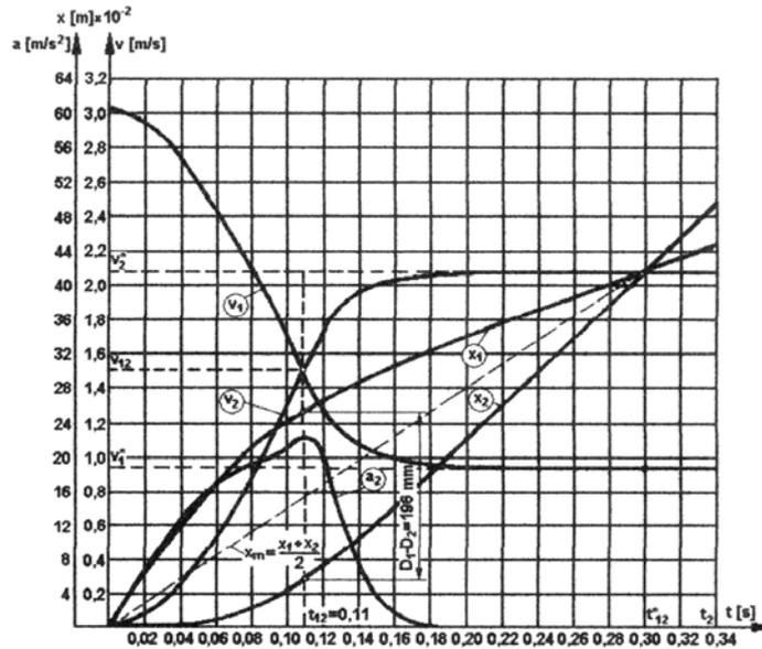
**Fig. 1** Time evolution of acceleration  $a_2(t)$  of collided car 2, determined experimentally and of the derived parameters  $v_1(t), v_2(t), x_1(t)$  and  $x_2(t)$  for collision  $C \rightarrow C$
