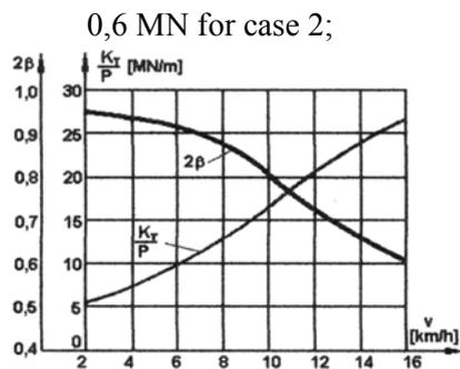
**Fig. 8.** The variation diagram of the  $2\beta$  factor and the  $K_T/p$  parameter, for the collision of two cars equipped with category A bumpers on the colliding car and category C bumpers (a solution of SC ICPVA SA) on the collided car
