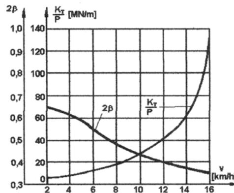
Fig. 7. The variation diagram of the  $2\beta$  factor and the  $K_T/P$  parameter, for the collision of two cars equipped with category A bumpers with rubber elastic elements (bumpers previously subjected to endurance testing)
