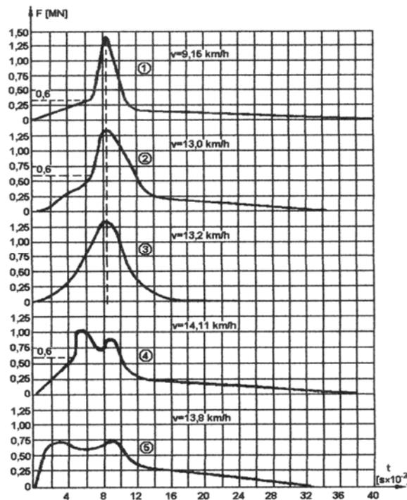
**Fig. 3.** The variation of the force transmitted through a bumper for different collision cases, depending on the type of bumper equipping the car and the collision speed  $v$ : 1 - 75 mm bumpers; 2 - category A bumpers with RINGFEDER rings; 3 - category A bumpers with elastic rubber elements; 4 - category A bumpers on the colliding car and category C bumpers on the collided car; 5 - category C bumpers.
