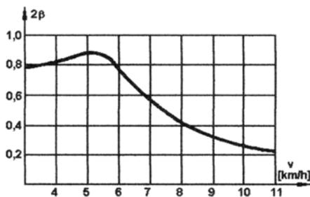
Fig. 4. The variation of  $2\beta$  according to speed, for the collision of two cars equipped with 75 mm bumpers
