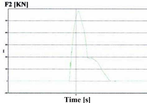
Fig. 17. Force transmitted to the car
