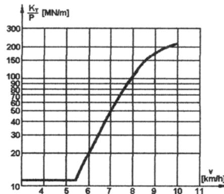
Fig. 5. The variation diagram of the  $K_T/P$  parameter according to speed, for the collision of two cars equipped with 75mm bumpers
