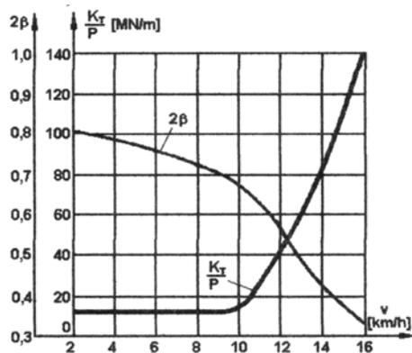
Fig. 6. The variation diagram of the  $2\beta$  factor and the  $K_T/P$  parameter, for the collision of two cars equipped with category A bumpers with the elastic element comprising RINGFEDER rings.
