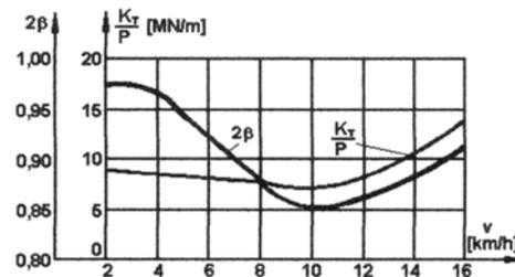
**Fig. 9.** The variation diagram of the  $2\beta$  factor and the  $K_T/p$  parameter, for the collision of two cars equipped with category C bumpers
