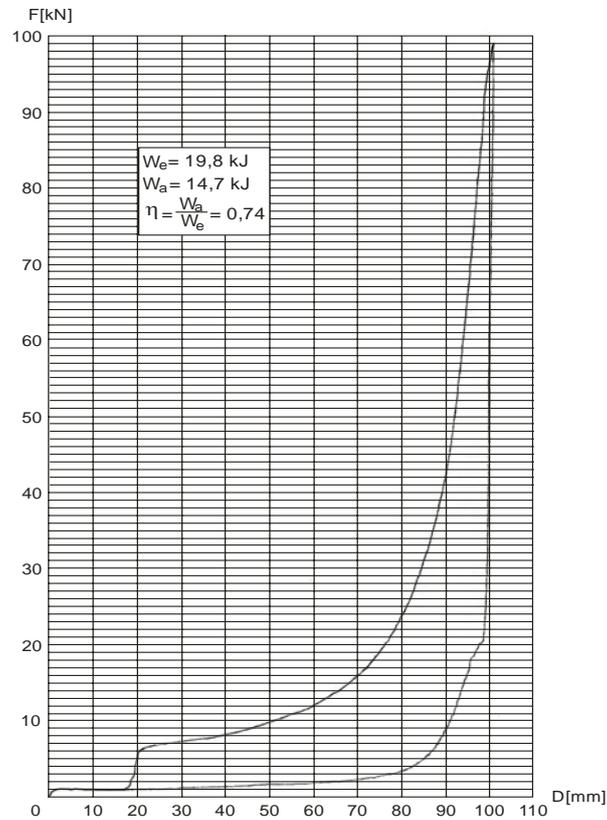
**Fig. 24.** Static diagram of the category C bumper used.
