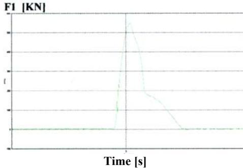
Fig. 16. Force transmitted to the car
