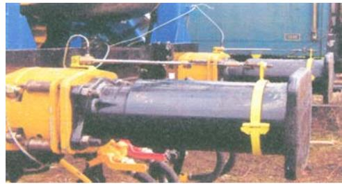
**Fig. 23.** D 3 - Coupling system displacement car A/car B
